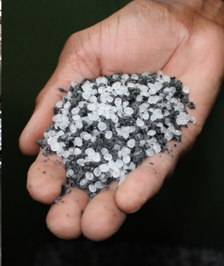
ABOVE FAR LEFT: Machinery is used to roll the tubing into wheel rims. ABOVE CENTRE: Plastic parts are manufactured from pebble-like plastic, which is melted down and moulded. ABOVE FAR RIGHT: The engineering room speaks volumes for the innovation, care and attention that goes into the CE Mobility chairs. RIGHT: The assembly line where the wheelchairs finally take on an recognisable form.
