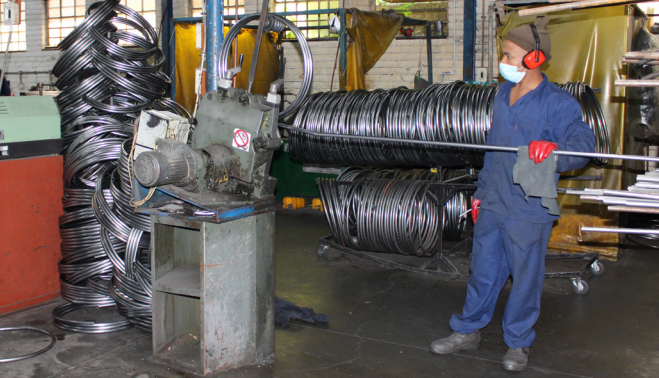
ABOVE FAR LEFT: Machinery is used to roll the tubing into wheel rims. ABOVE CENTRE: Plastic parts are manufactured from pebble-like plastic, which is melted down and moulded. ABOVE FAR RIGHT: The engineering room speaks volumes for the innovation, care and attention that goes into the CE Mobility chairs. RIGHT: The assembly line where the wheelchairs finally take on an recognisable form.
