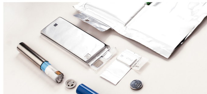
From the left: two cylindrical cells (one open and one closed), two pouch cells, a coin cell and a large pouch cell.
