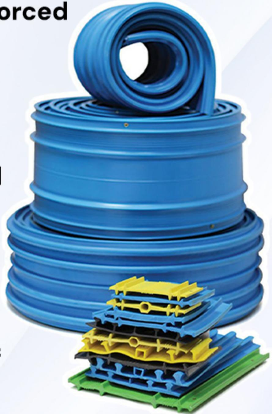
**The many sections centrally and externally placed allow lasting watertight seals in any grades of concrete design; the cross section configuration features a multi rib design for an effective grip and tenacious anchor to the concrete and a flexible, hollow center bulb to accommodate moderate expansion and contraction in the concrete joints.**
