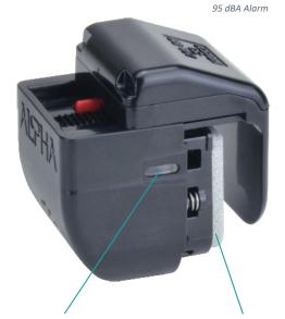
Flashing LED provides strong visual deterrent
