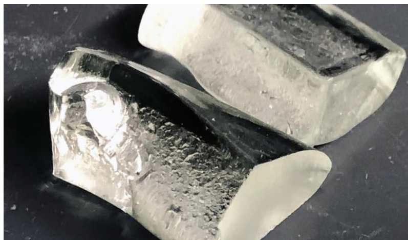
A sample of LionGlass, a new type of glass engineered by researchers at Penn State that requires significantly less energy to produce and is much more damage resistant than standard soda lime silicate glass. Credit: Adrienne Berard/Penn State
