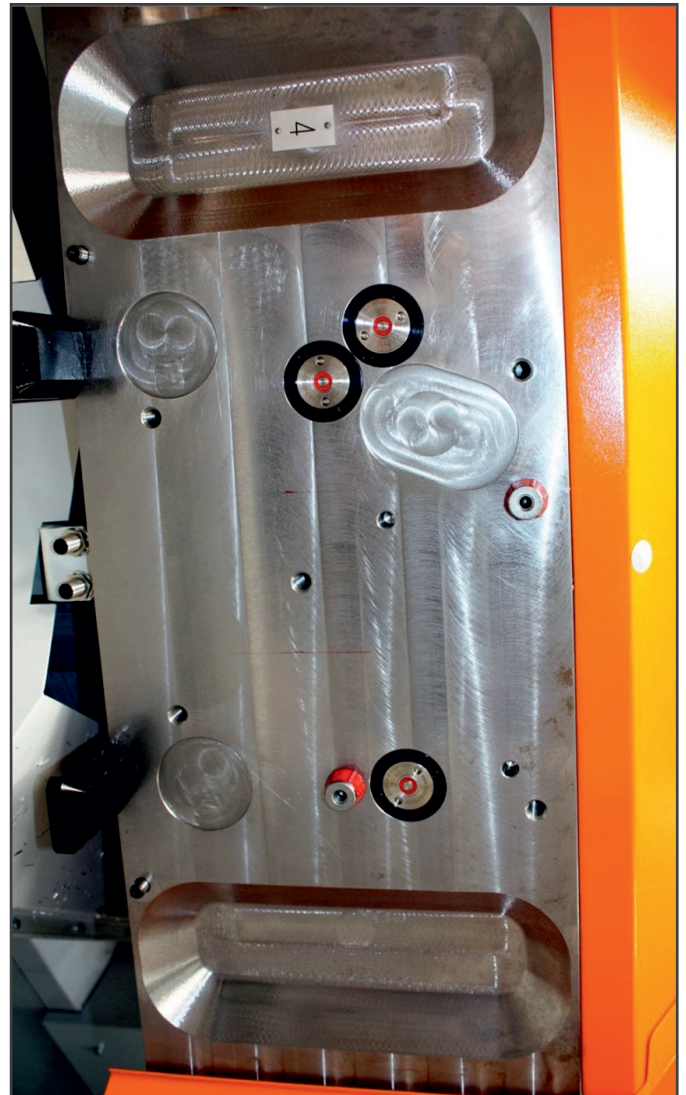
The base body of the change fixture contains coupling for automatic opening and closing of the hydraulic supply during the loading and unloading processes
