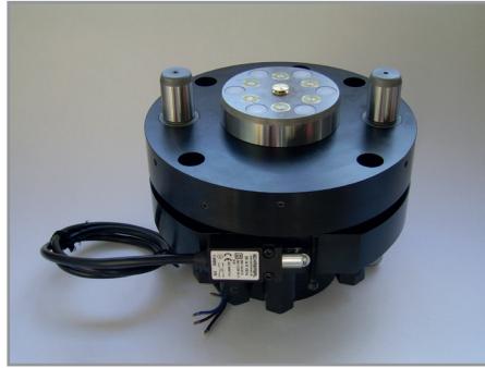
Docking station with six coupling points, pressurized coupling; in order to dock the coupling plate, it is raised by an integrated hydraulic cylinder.
