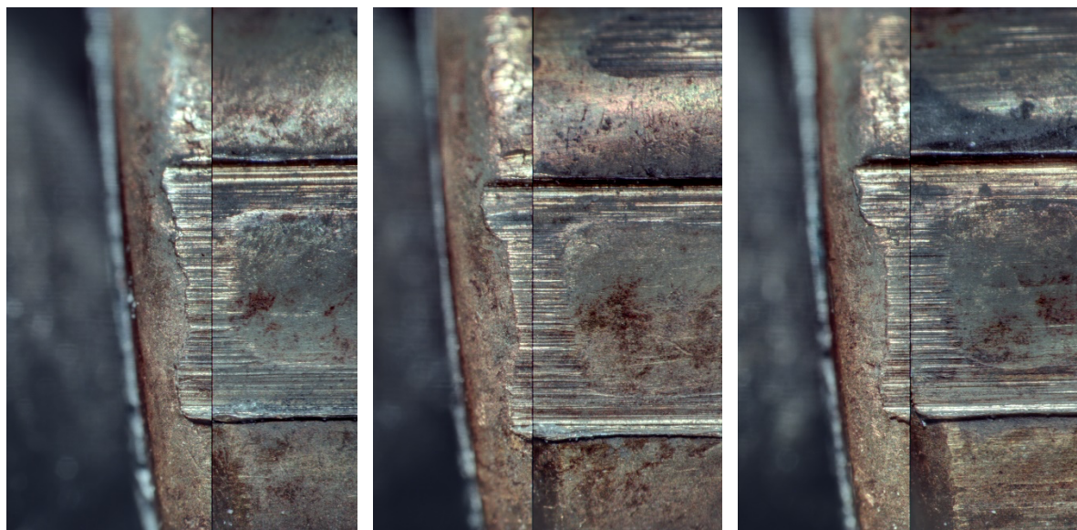
Figure 5: Three different land-engraved areas of TF-01-A and Unknown 3 using VisionX
