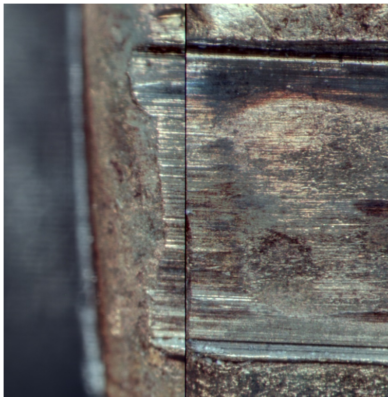
Figure 23: Correspondence observed between bullets from different sources
