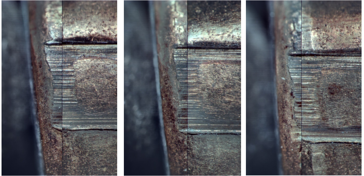
Figure 6: Three different land-engraved areas of TF-02-B and UNK-14 using VisionX
