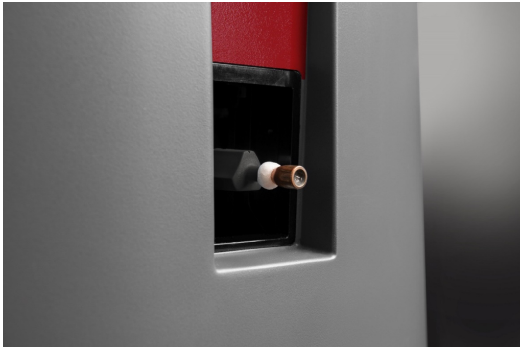
Figure 3: Bullet mounted prior to acquisition into the Q3M
